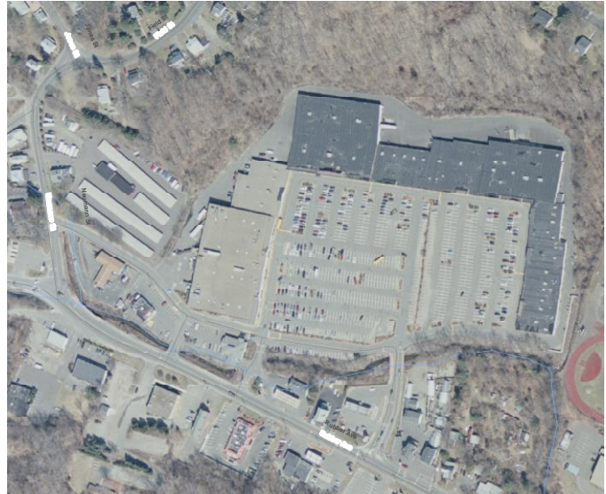
Figure 3. Aerial photograph of mall on Rubber Avenue near Neumann Street. Gray and black areas are impervious asphalt, which in this area cover perhaps 70% of the watershed surface, up to the very edge of the brook channel. Rain falling on this area quickly drains into storm sewers and then into the brook.
