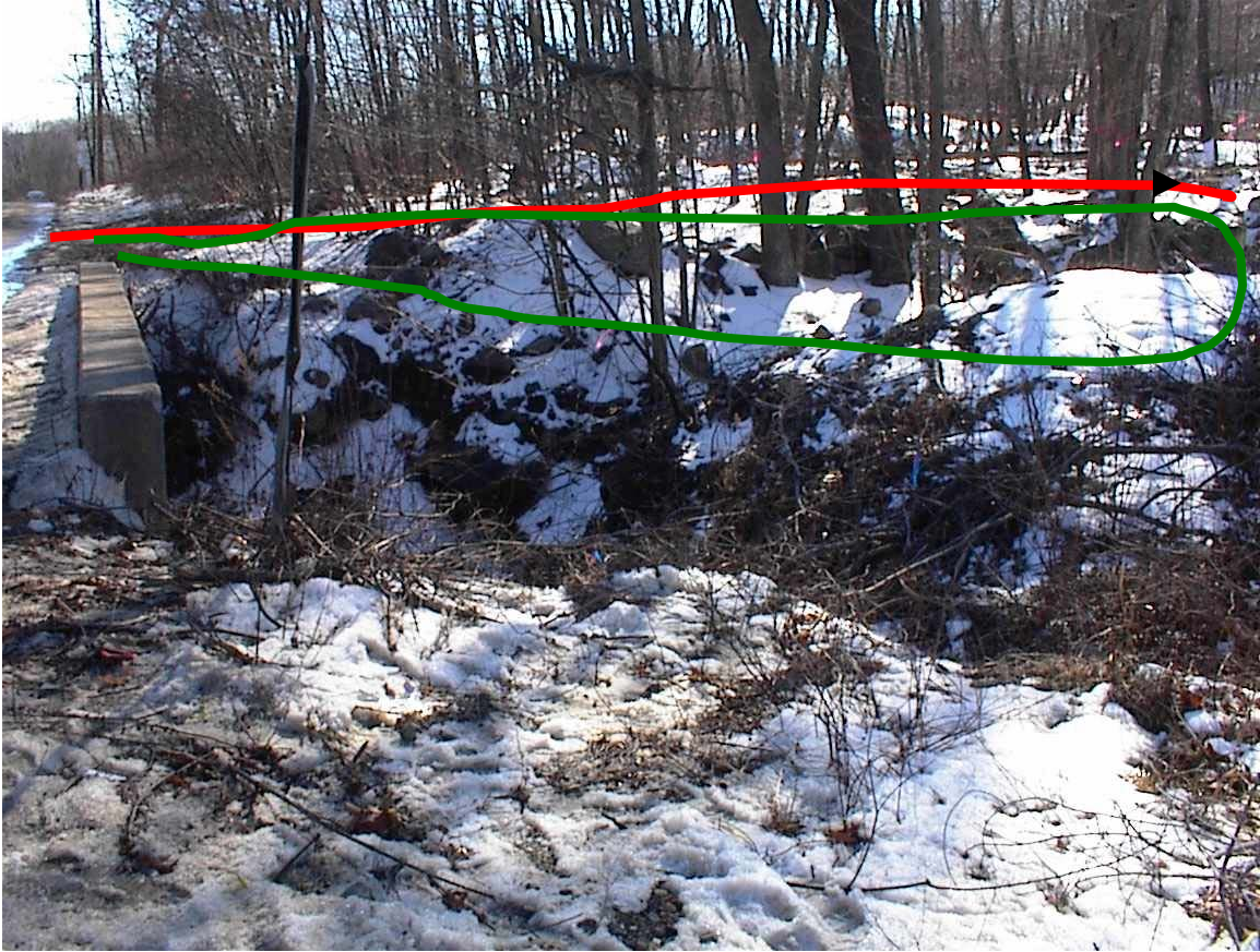
Photo Six: Looking South at Highland Avenue stream crossing. Red line is approximate location of proposed access road to project. 10 feet minimum of natural vegetation should remain between top of bank and disturbance for road. The stormwater treatment structure should be on the streamside of the proposed road to make the open area contiguous and to provide a buffer from road use.
