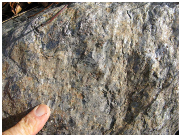
Figure 6. Littleton Formation consists of gray mica schist, some of which is garnitiferous. Mica grains are microscopic but give the rock a silvery sheen. Long and narrow black rectangular grains are staurolite.
