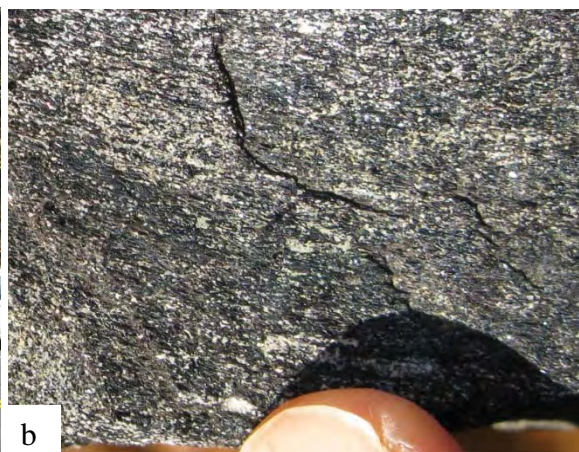
Figure 3. Fragments of Brimfield Schist that are part of the dam for Lower Bolton Lake. They contain iron sulfide minerals that weather by dissolving and releasing iron oxide and sulfuric acid to the environment. Iron oxide is precipitated almost immediately in an oxidizing environment. Note on the right that what was originally a rock fragment is now rubble. Disc on key-chain in both images is 2 inches in diameter.
